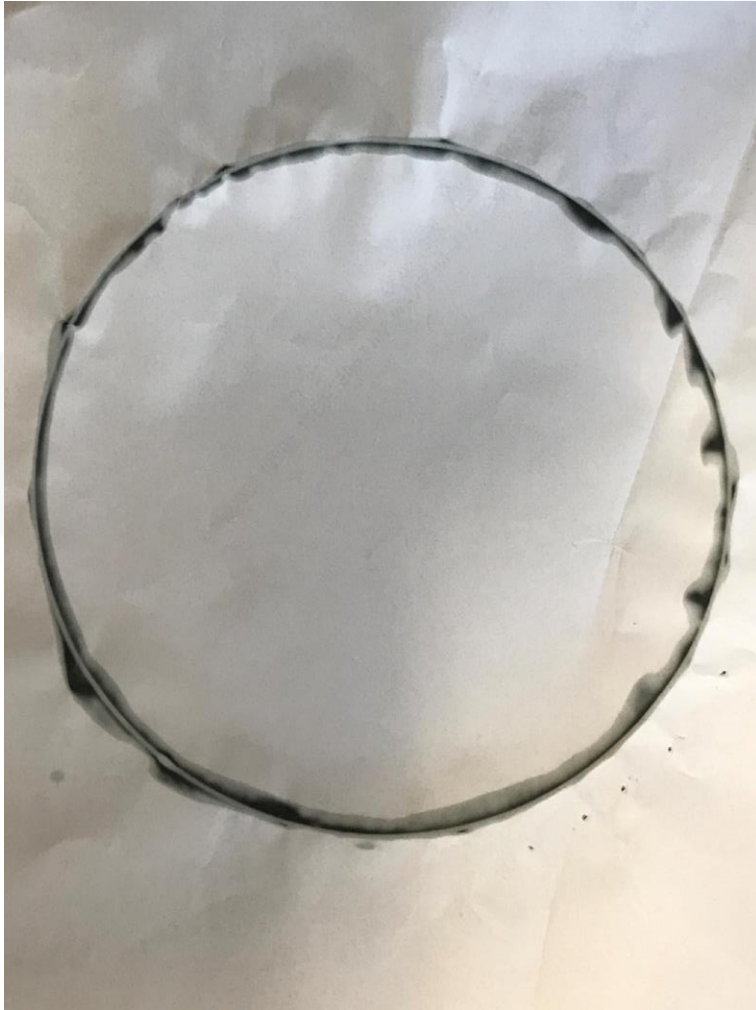
Impression Paper- a tool to check seal uniformity
